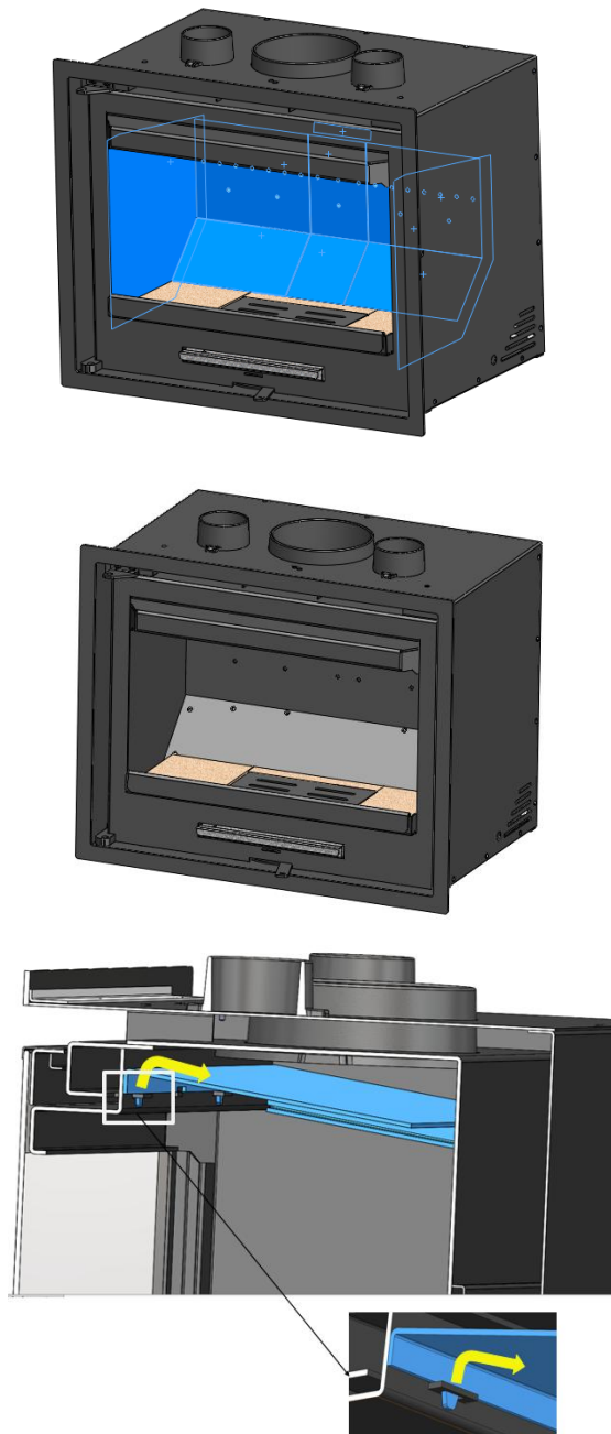
Figure No.9 - Dismantling the ADOUR steel deflector
