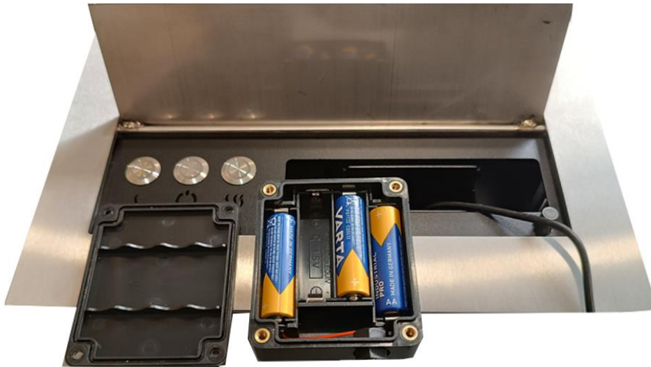
Fig. 11 – Putting back the battery box
