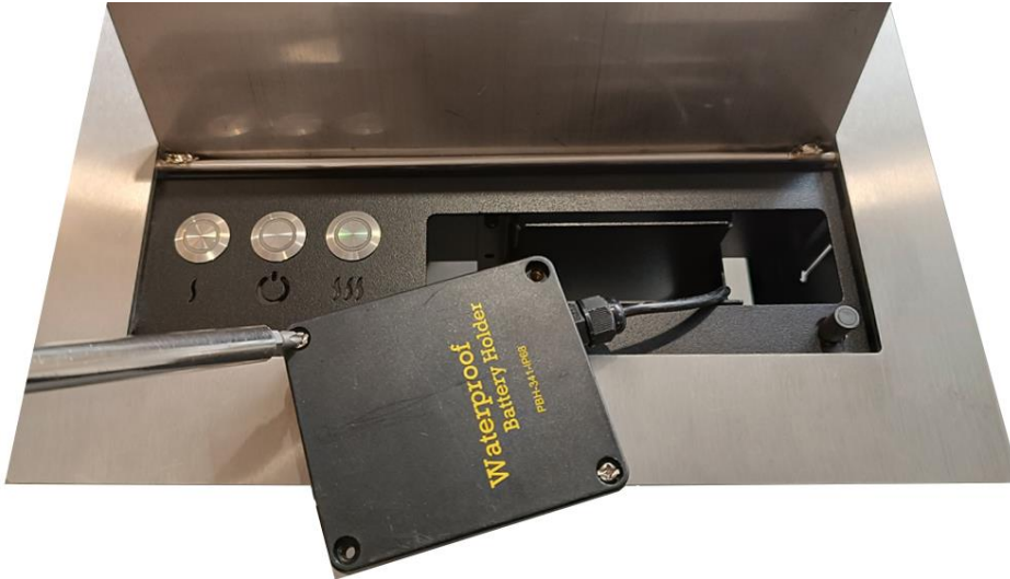
Fig. 10 – Replacing the batteries in the container
